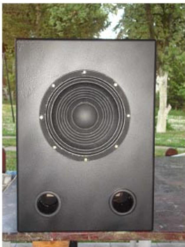
NISKOFREKVENTNA AKTIVNA ZVUČNA KUTIJA SLUŽI ZA REPRODUKCIJU TONOVA NIŽIH FREKVENCIJA ( DO 100 Hz ). KVALITETNA REPRODUKCIJA NIŽIH TONOVA DOLAZI DO IZRAŽAJA KOD SLUSANJA GLAZBENOG MATERIJALA SA FILMOVA.
